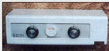
G3EAY finds that the high-impact plastics case of a discarded toaster (top) can be transformed into a housing for an antenna tuning unit, etc (bottom).
